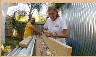
Use the hand planer to flatten the edges of your planks as best as possible. We started with three, 6 inch wide planks and had them cut lengthwise into six, 3 inch wide ones.
