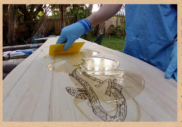
The last step is to coat your board either with traditional linseed oil or some type of resin. We strongly advise using a resin. This will strengthen your board substantially, which us kiters need! We've also begun experimenting glassing our boards, but that is a tale for another day....
