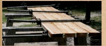
Using as many clamps as you can acquire, coat each plank edge with epoxy (add filler to thicken the resin) and carefully squeeze the planks together.
