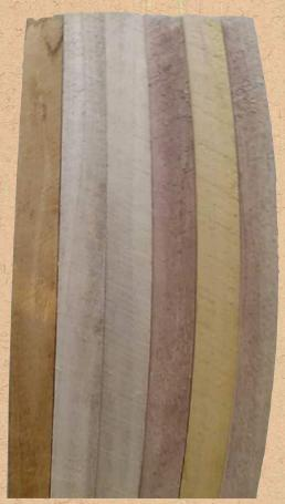
Make your own blank out of planks. Use 1 inch thick planks, the width is up to you
