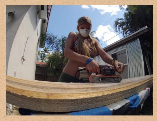
If you've made your own blank, you'll want to use a belt sander and remove material until the board has uniform thickness of about 0.75 inches. The better you do this, the easier the rest of the building process will be.
